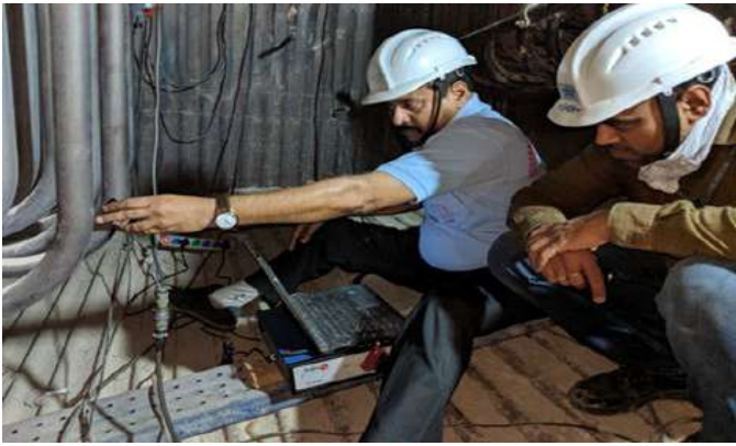
Detection of Magnetite at tube bend
