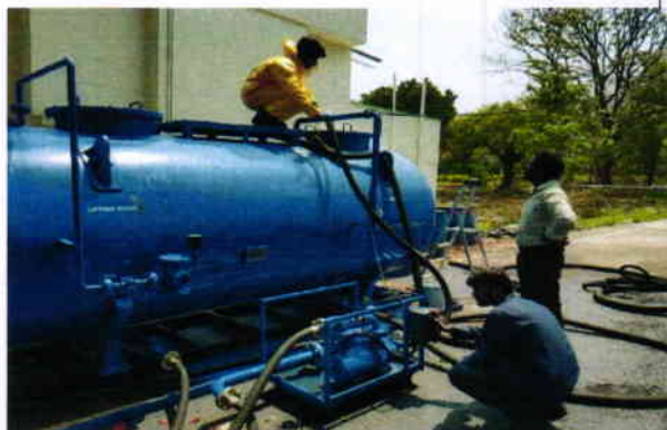
Fig.8: PCB staff members loading transformer oil to reactor through inlet hose pipe of PCB de-chlorination unit.
