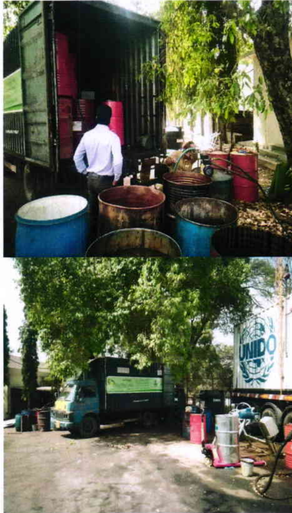
Fig.12: Loading of PCB de-chlorinated oil and sludge to the vehicle of M/s KarRecycle Centre LLP, for disposal.
