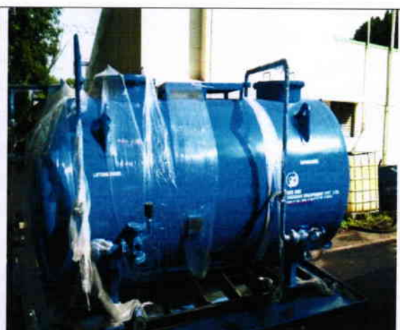
Fig.6: PCB contaminated oil stored in 6kl MS tank
