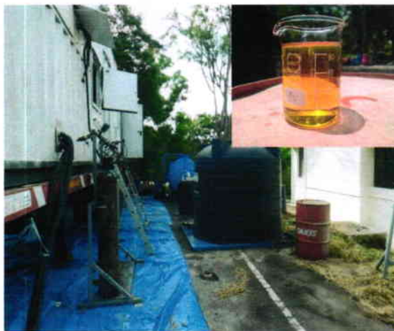
Fig.11: Oil after PCB de-chlorination stored in 5KI Plastic tank for disposal
