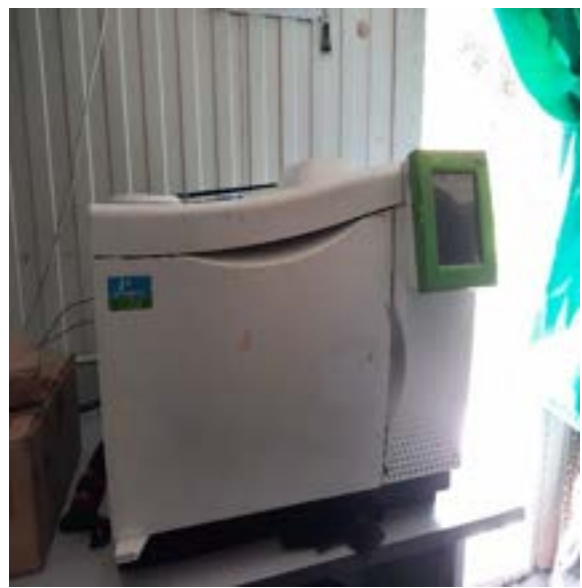
Figure 25: GC-ECD instrument used for PCB analysis
