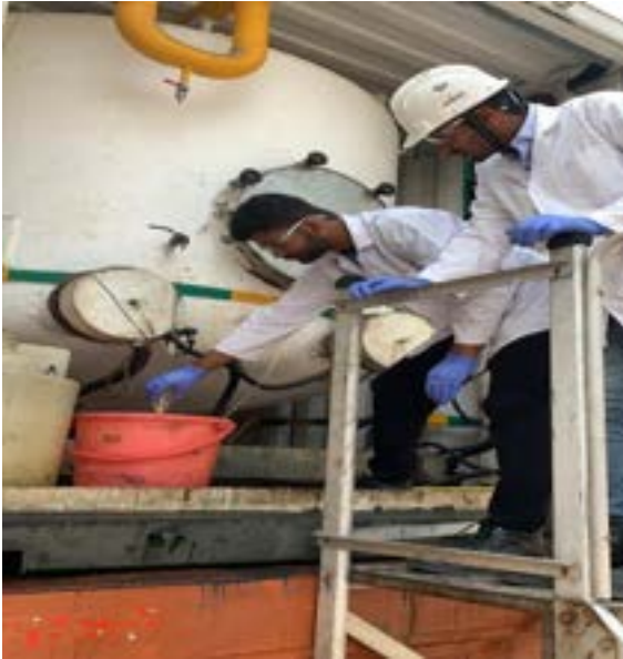
Figure 30: Sample is collected for PCB analysis
