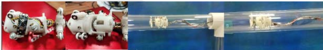
Figure5. Travelling of robot in 50mm dia. pipe remotely along with lidar sensor.
