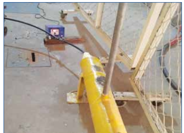
Water Penetration Test for Medium Voltage Covered Conductor (MVCC)
