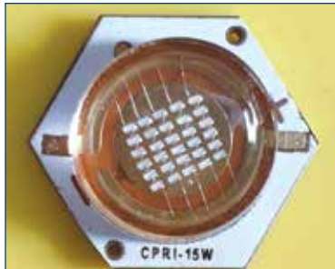
A prototype of chip on board LED package
