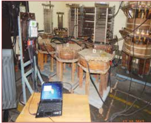
Smart Meter under Load Switching Capability test
