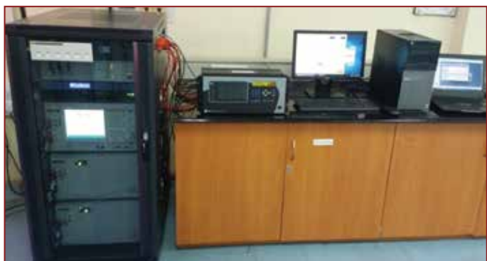
6135A PMU Calibrator Test facility
