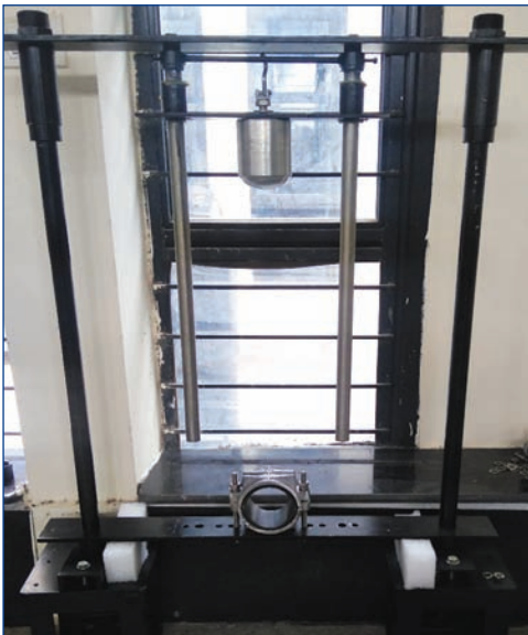
Vertical drop impact tester
