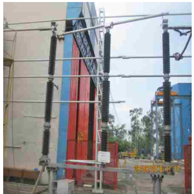
Short time withstand current and Peak withstand current test at 63kArms for one second with initial peak of 158kA as per Clause 6.6 of IEC: 62271-102, 2001 on 420 kV , 3150A Horizontal Double Break Disconnecter carried out at STDS-CPRI, Bhopal for GR Power Switchgear Limited, Hyderabad
