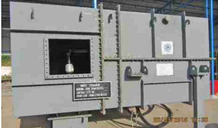
Short time current test conducted on Terminal Box for M/s. Skipper Seil Ltd., Bhiwadiat STDS-CPRI, Bhopal
