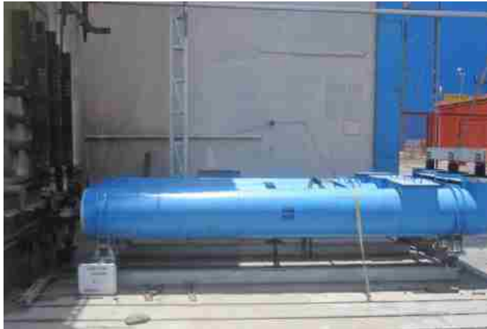
Short time withstand current test at 90kArms for one second with initial peak of 230kA as per IS: 8084 on 11 kV , 4000A, 90kArms Busduct for M/s. BHEL, Rudrapur carried out at STDS-CPRI, Bhopal
