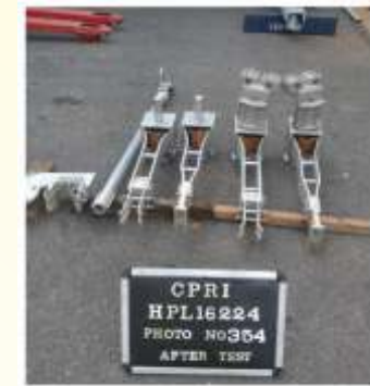
123 kV Center brake disconnecter of M/s. Centaur switchgear, Chennai was tested for short time withstand current test of 31.5 kA for 3 sec.
