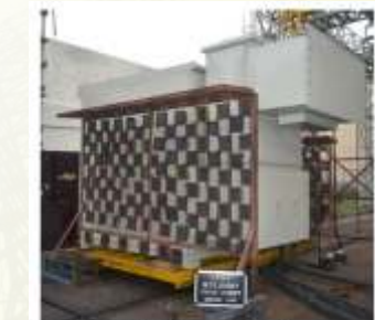
36 kV, 25 kA, 1250A Metal enclosed switch gear & control gear of M/s. Toshiba T&D systems India Pvt Ltd., Hyderabad was tested for internal arc test of 20 kA for 0.1 sec.
