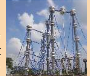
HVDC Generator at UHVRL, Hyderabad
