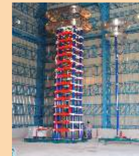
2400kV, 240kJ Impulse Voltage Generator
