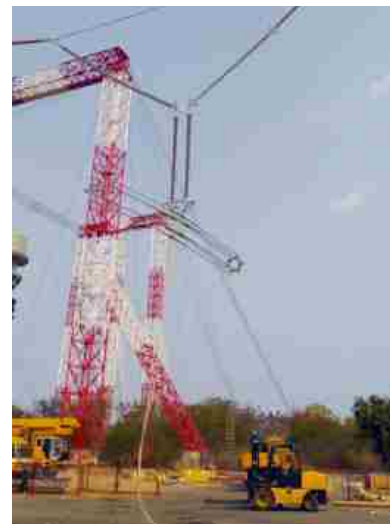
Lightning Impulse voltage withstand test and Wet Switching impulse voltage withstand test on \pm 800 kV HVDC Single "Y" suspension Composite long rod insulator string for M/s. Deccan Enterprises Ltd., Hyderabad
