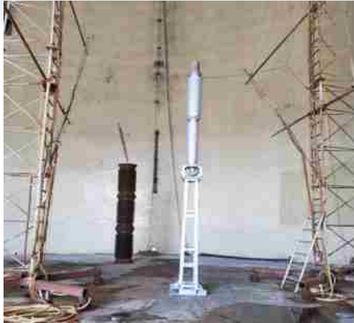
Pollution test on 145 kV, 2000A, Single pole Circuit Breaker with composite insulator housing carried out at UHVRL-CPRI, Hyderabad for M/s. Siemens Limited, Aurangabad
