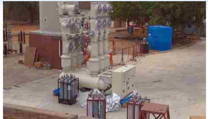
Lightning Impulse voltage withstand test and Switching Impulse voltage withstand test conducted on 420kV, GIS for M/s. Siemens Limited, Aurangabad at UHVRL-CPRI, Hyderabad
