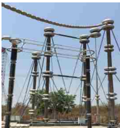
DC RIV test and DC corona test conducted on \pm 800 kV, Spacer damper with retaining rods for six bundle lapwing ACSR conductor for M/s. EMI Transmission Limited, Mumbai at UHVRL-CPRI, Hyderabad
