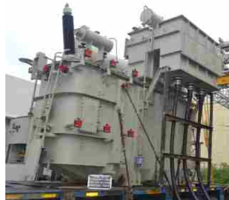
Ability to withstand the dynamic effects of short circuit tests on 25 MVA, 110/33 kV, three phase transformer carried out at High Power Laboratory, CPRI, Bangalore, for M/s. Transformers & Rectifiers Ltd., Ahmedabad
