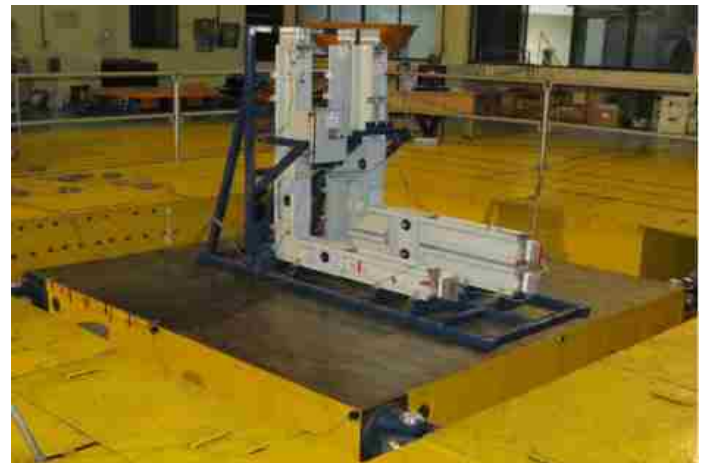
Seismic test on Sandwich Busway System – Guardex for M/s. RR Busduct Power Distribution Equipment, Dubai carried out at Earthquake Engineering & Vibration Research Centre, CPRI, Bangalore
