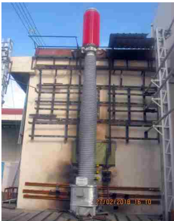
Short time current test at 50kArms for three seconds with initial peak of 125kA on 800kV, 500-1000-2000-3000/1-1-1A, Current Transformer for M/s. ABB India Ltd., Vadodara
