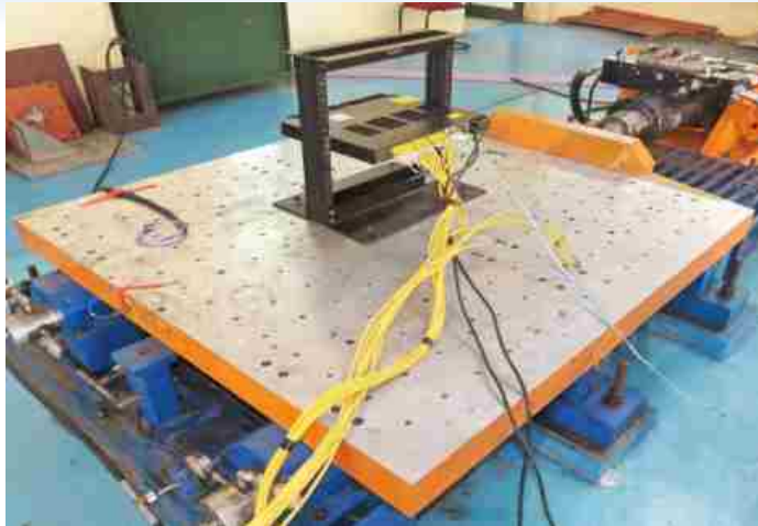
Vibration tests on 250 W Power supply unit inserted in the IE 5000 series switch carried out at Earthquake Engineering & Vibration Research Centre, CPRI, Bangalore for M/s. Integrity Electronics LLC, Apopka, FL 32703
