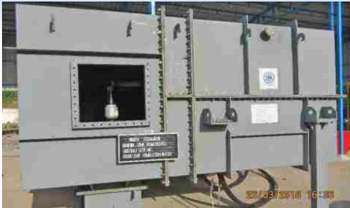
Short time current test conducted on Terminal Box for M/s. Skipper Seil Ltd., Bhiwadiat STDS-CPRI, Bhopal
