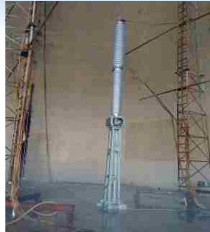
Pollution test by salt-fog method on 245kV, Single pole Circuit Breaker with composite insulator for M/s. Siemens Ltd., Aurangabad carried out at UHVRL-CPRI, Hyderabad
