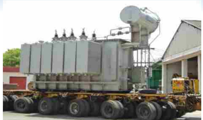
M/s. Energypac Engineering Ltd, Dhaka-1208, Bangladesh has conducted temperature rise test on 20/28 MVA, 33/11.5 kV Power transformer at 25kA Temperature rise Lab, Bhopal.
