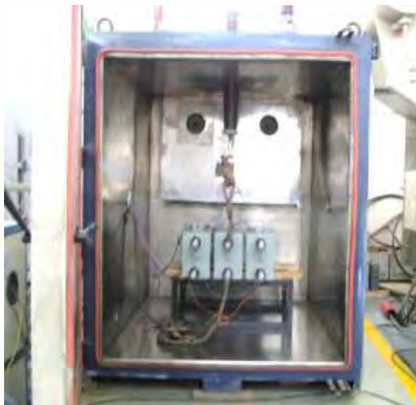
Arrangement for Thermal Stability Test on 1100kvar, 7.3kV, 68 \mu F Internal Fuse capacitor unit
