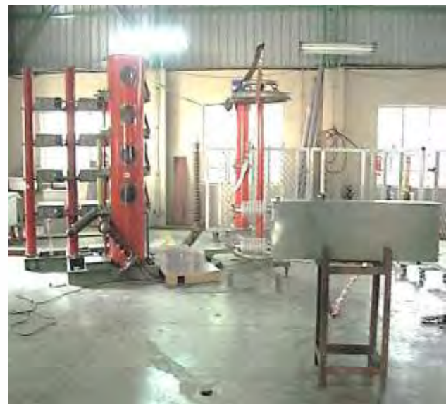
Arrangement for Lightning Impulse voltage test on 1000kvar, 22kV, 6.9 \mu F Fuseless HT capacitor
