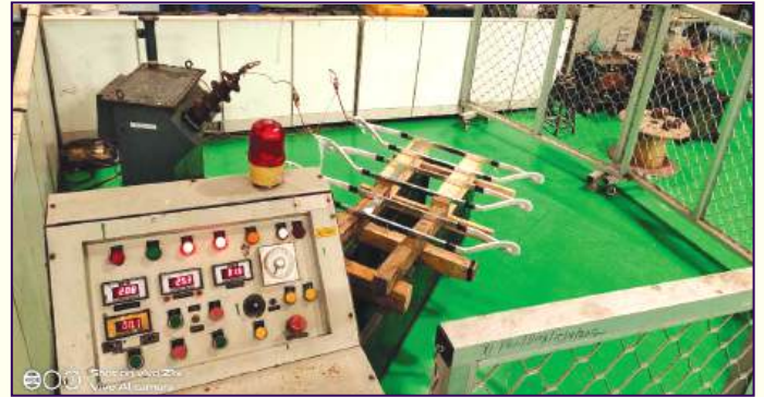
Setup for Voltage Endurance Test on Stator Coils
