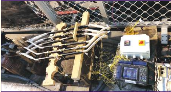
Test setup for Thermal Cycle Test on Stator Coils
