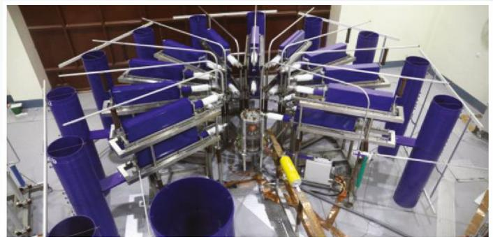
100 kV, 300 kJ Impulse Current Generator
