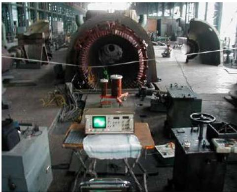
**Partial Discharge test on
