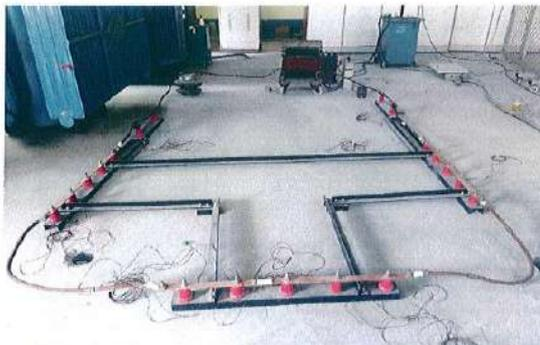
Fig 1: Test Set up for Heating Cycle Test
