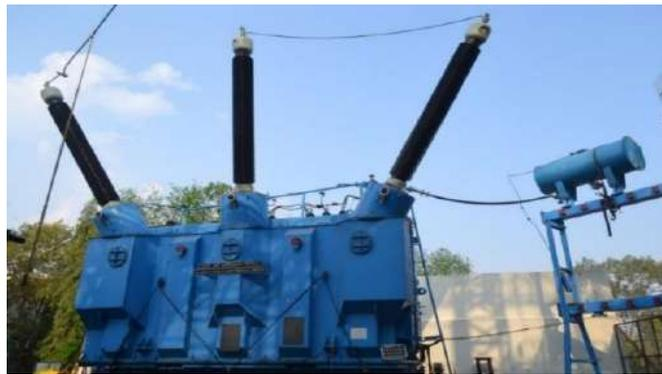
**Ability to withstand the dynamic effects of short circuit test on 100 MVA, 400/11.5-11.5kV three phase transformer**
