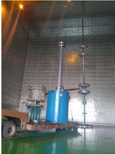
**800KV RIP Transformer Bushing undergoing Partial Discharge test**
