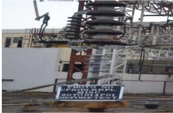
**Power Arc test on 25kV composite insulator**
