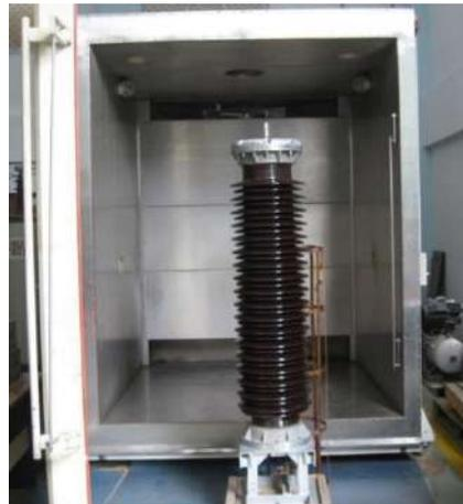
**A view of the 170 kV, 4400pF capacitor module of CVT**
