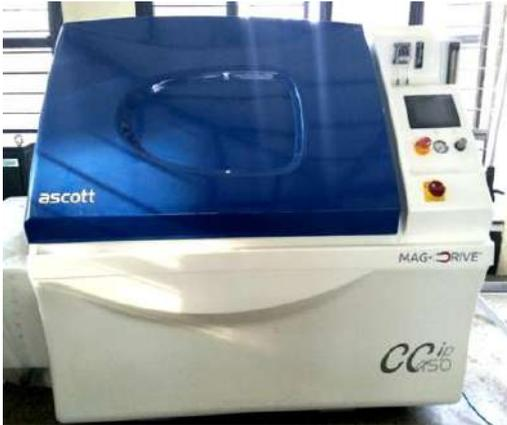
**Cyclic Corrosion Test Equipment**
