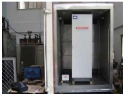
**Test arrangements for the testing of the BHELSONIC-Acoustic steam detection system**
