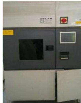
**Weathering using Xenon Arc Lamp**
