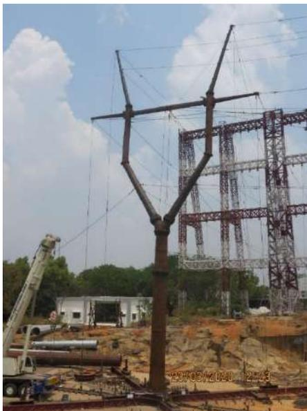
Testing of 400 kV S/C “Y” shaped steel monopole
