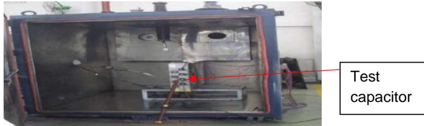
**A view of the test capacitor on completion of the destruction test**
