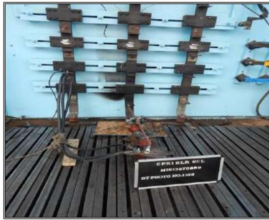
Short-time current test on Ground Clamps
