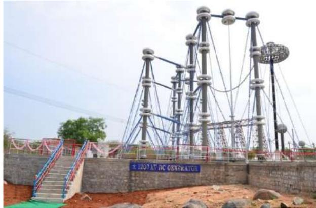
A View of ± 1200 kV DC Test System
