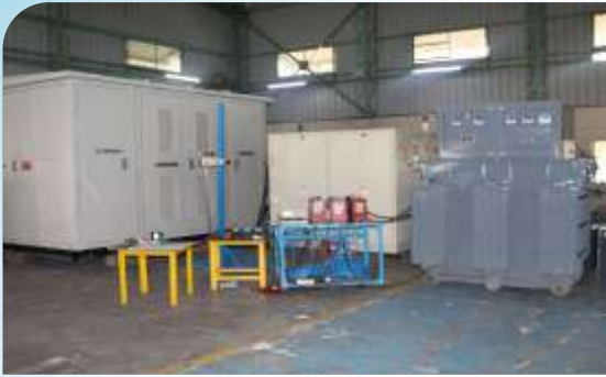
Continuous current test on Compact Substation of 2MVA, 11kV/433 V with Dry type Transformer
