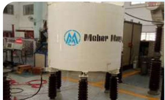
Temperature rise test on air core, dry type, 1Ø, 33/√3 kV, Filter Reactor
