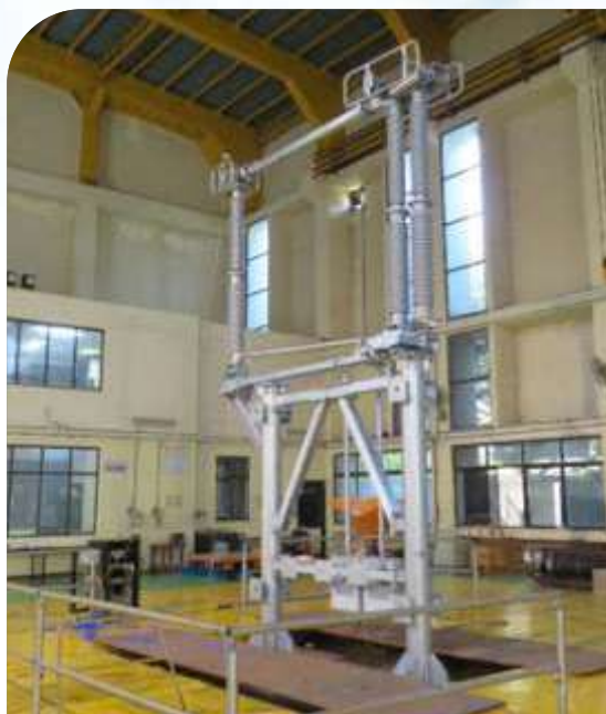
Seismic test on 362 kV, Vertical Break Disconnecter with grounding Switch
