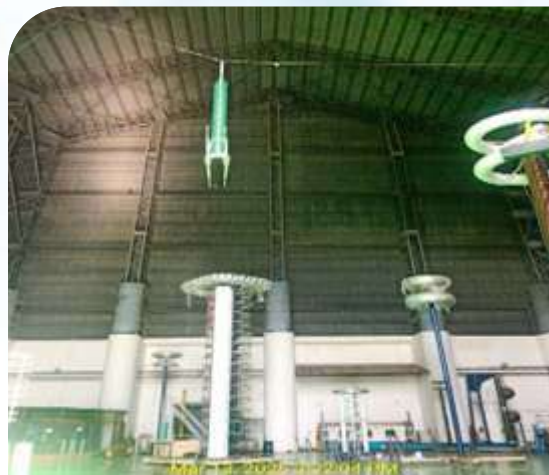
Chopped Impulse Voltage test on Link Box 3/1 and 6/1 suitable for 132kV and 400kV Cable System
