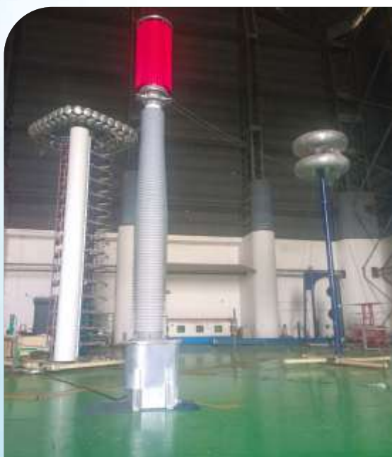
Multiple Chopped Impulse test on 765kV Current Transformer with 600 application of chopped impulse at 1680KVp
