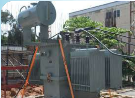
Dynamic and thermal Short Circuit test on 1250 kVA, 11/0.415 kV Distribution Transformer
