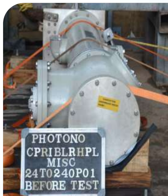
Short time withstand current test at 50kA rms for 3.0 s on 245 kV Gas Insulated Line used in GIS application
