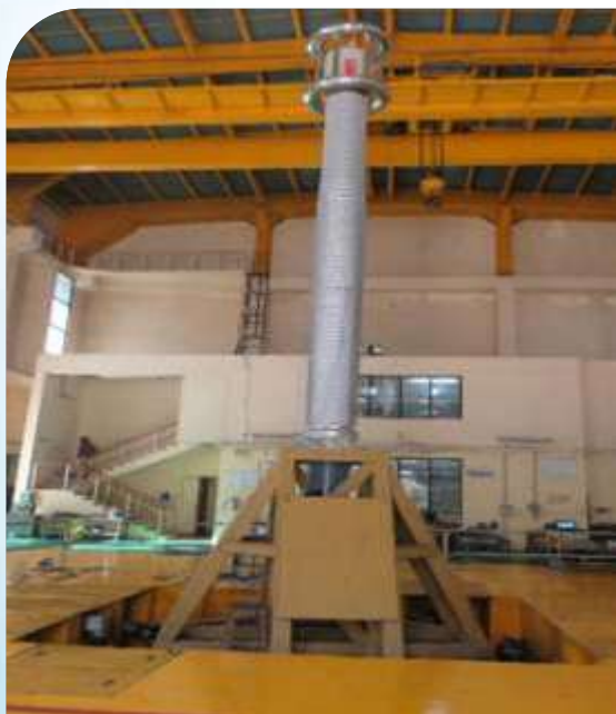
Seismic test on 800 kV Transformer Bushing
