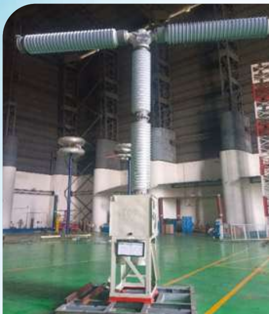
Lightning Impulse and Switching Impulse tests on 420kV SF6 Gas Circuit Breaker using two Sources (Combined Voltage Test)
