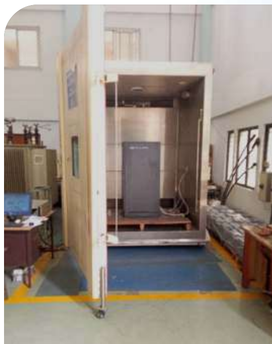
Environmental testing on 1Ø, 20 kVA, 20kW, 230Vac, 50 Hz UPS
