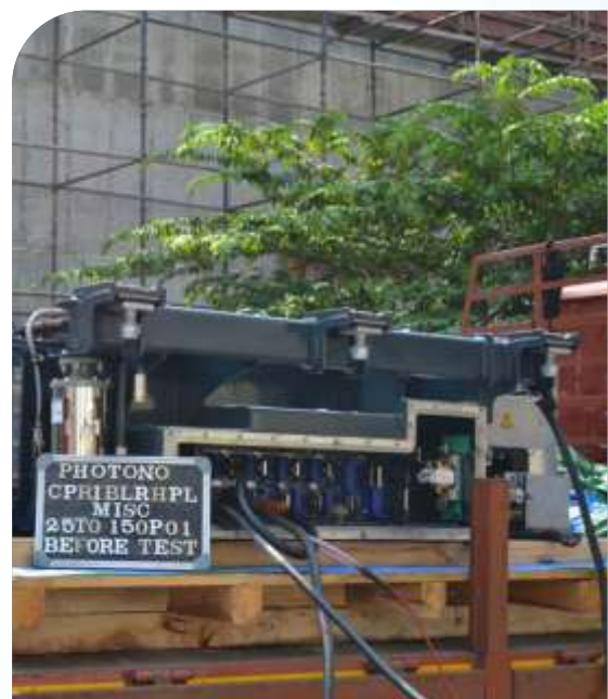
Dynamic Short Circuit test and inrush current measurement test on 2400 kVA, 25 kV Traction Transformer
