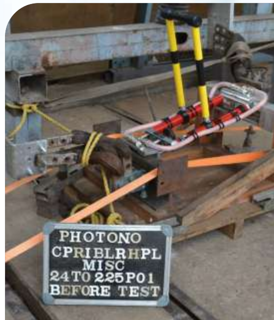
Short time withstand test on Rail earthing system for 105kA, 40 milliseconds
