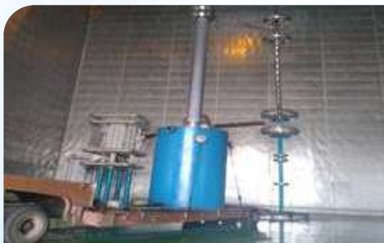
800kV RIP Transformer Bushing under Partial Discharge test
