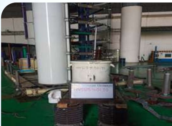
Chopped Impulse Voltage test on 5kVA and 25kVA, 6.35/0.240kV, Single Pole Distribution Transformer
