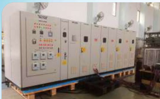
Test arrangement for testing of 6.6 kV, 4000 kVAR, 3 Ø, 50 Hz, MV APFC Panel
