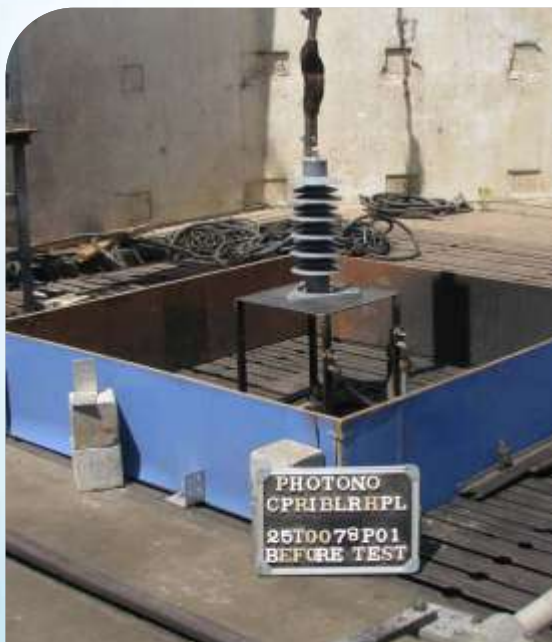
Short circuit test at 63kA on 42kV/10kA Polymer Surge Arrester
