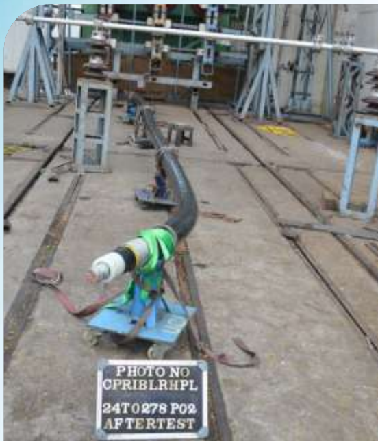
Short time withstand current test on Cable Sheath of 220kV XPLE Cable
