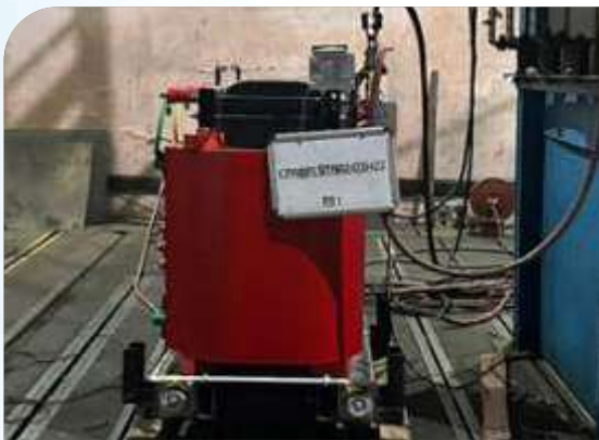
Routine test on 2500 kVA, 11/0.415 kV, Three Phase, Cast Resin Dry Type Distribution Transformer
