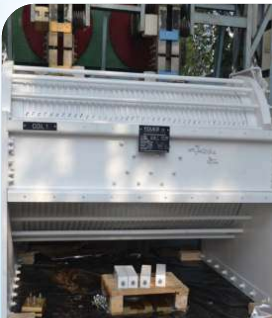
Dynamic short circuit test on Short Circuit Current Limiting Reactors
