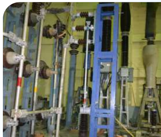
Short Time Current test on 12kV & 36kV Single Pole Neutral Disconnecter
