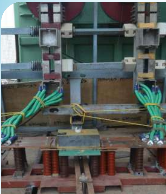
Short-time withstand current at 100kA for 3s & 250kA peak on High Current Measuring Shunt
