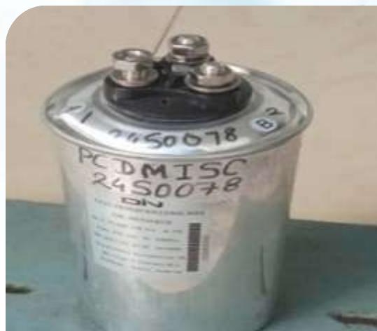
A view of 3 x 40µF, 850 VAC, 50 Hz, AC capacitor, Self-Healing Type, Aluminium cylindrical, Power Electronic Capacitor for Solar application
