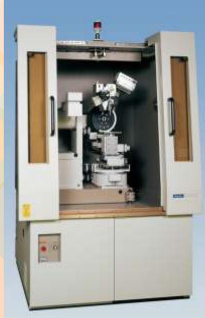
*Residual stress test - XRD based*
