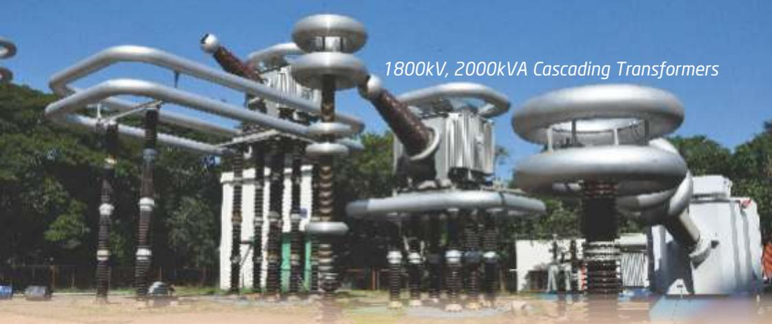
1800kV, 2000kVA Cascading Transformers
