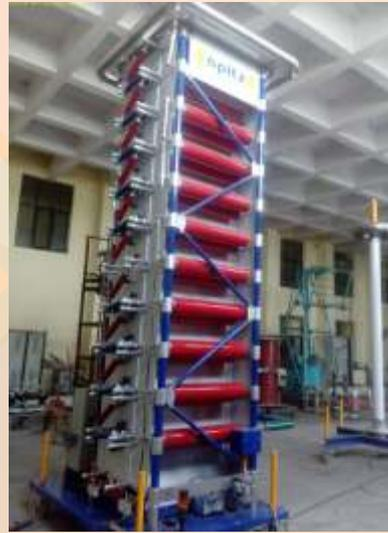
*1000kV, 100kj Impulse Voltage Generator*
