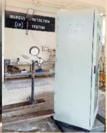
**Ingress Protection Testing Laboratory:** The lab is equipped with dust test chamber to perform IP 5X and 6X to accommodate the test panels/ samples of size up to 2.2 m x 1.8 m x 2.5 m (W x L x H) and water test facility to perform tests ranging from IP X1 to X8 test. The Lab undertakes the tests ranging from IP 11 to IP 68.
