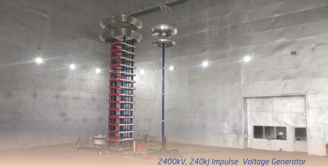
*2400kV, 240kJ Impulse Voltage Generator*
